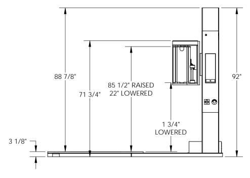
\*115V SUPPLY VOLTAGE; INCLUDES POWER CORD WITH NEMA 5-15 PLUG \*10A AT FULL LOAD
