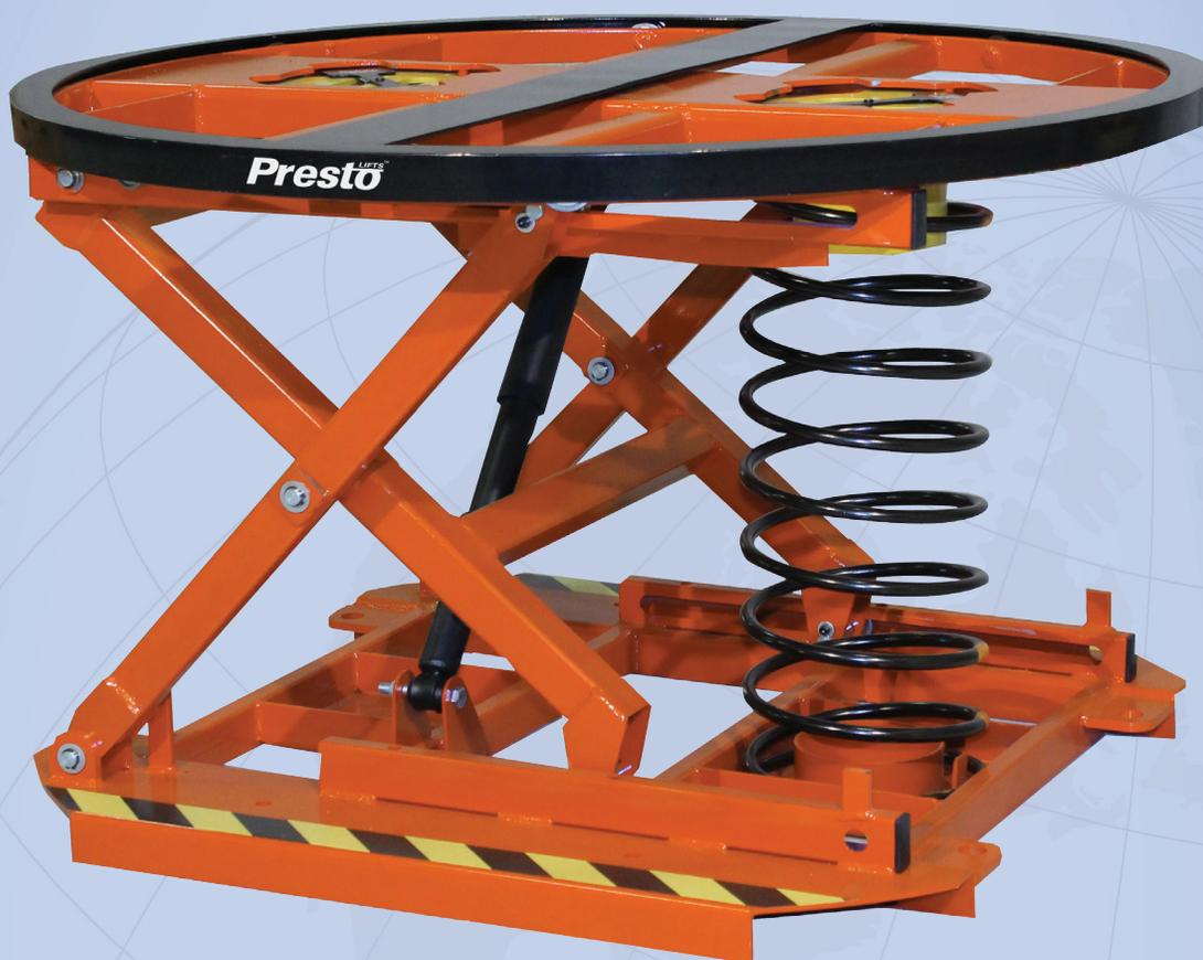
The P3-Spring Level Loader improves the efficiency of manual pallet loading and unloading jobs by eliminating bending, stretching, and walking around the pallet. Heavy-duty springs and shock absorbers lower or raise pallets as boxes are added or removed. An anti-friction turntable top lets workers stand in the same position throughout the loading and unloading process.
