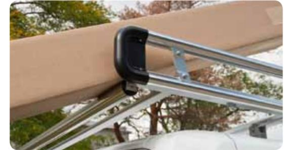
Rear Roller makes loading and unloading easy
