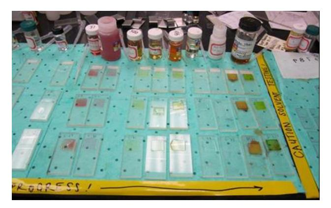
The results of the water contact angle testing are as follows. Shown are the control (untreated glass slides) and the slides treated with Gentoo:
