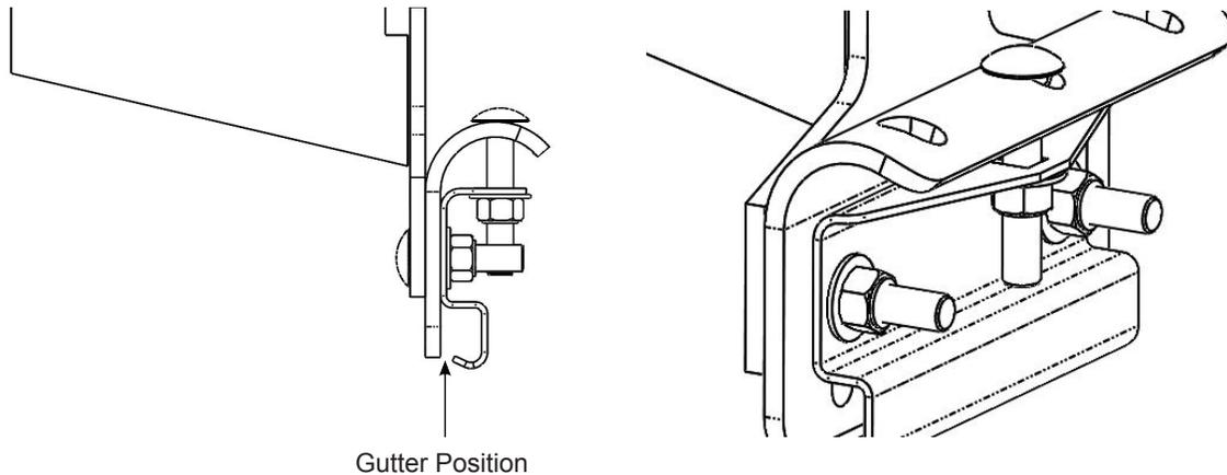
Position the cross member to desired position and tighten the two nuts to 17 ft-lb. Vertically constrain the inverted J-bracket and the gutter clamp using one 1-3/4" carriage bolt, washer, and a nut.
