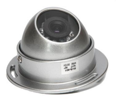
This 92° dome camera is great for indoor monitoring as the camera is a forward facing view. The dome camera boasts a 250,000 pixel 2.1 mm lens with 9 infra-red illuminators which enable you to see in total darkness. The casing of the camera has an IP65 rating which can withstand minor weather conditions. The camera includes a 26' weatherproof cable with has a 4 pin S Video connection.
