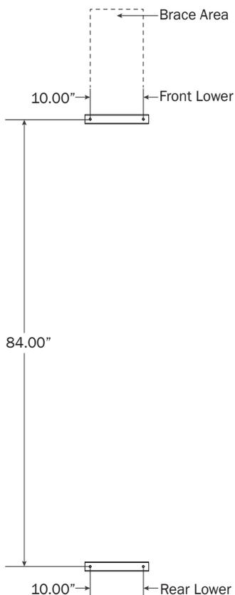
**0.3** 8.00 Ft: Drill holes into the Service Body mounting location according to dimensions shown.
