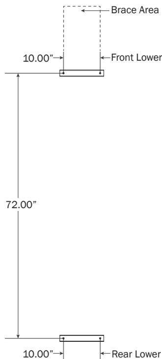
**0.2** 7.00 Ft: Drill holes into the Service Body mounting location according to dimensions shown.
