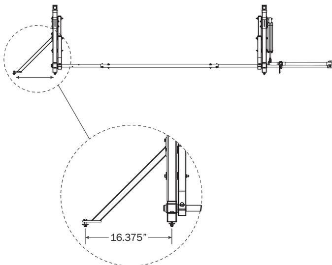
**0.1** 6.00 Ft: Drill holes into the Service Body mounting location according to dimensions shown.
