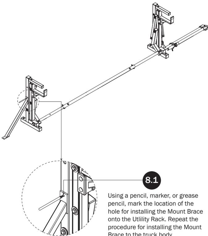
**8.2** Remove the Mount Brace to expose the bolt hole markings. Using a 9MM, 23/64", or T size bit, drill a hole into the Utility Rack at the marked bolt hole location created during Step 8.1.
