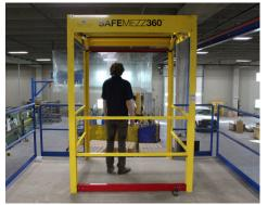
▲ DANGER Never operate SafeMezz360 within the pallet drop area when the edge is exposed. Incorrect operation shown.
