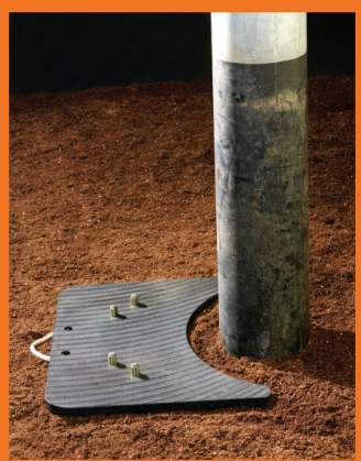
Place pole puller pad around the pole.
