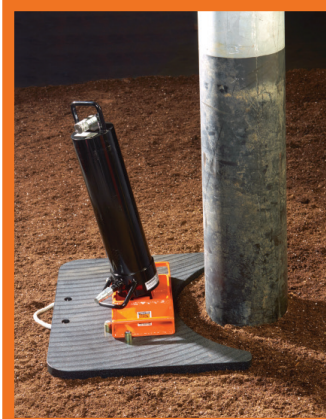
Set the hydraulic cylinder onto the base plate.
