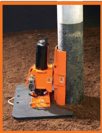
Attach the steel clamshell to the swivel.
