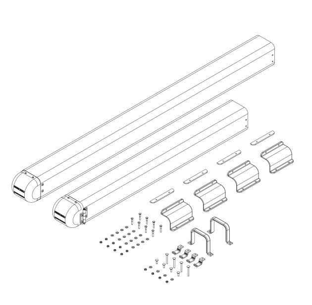
SPLICED CONDUIT TUBE ASSEMBLY
