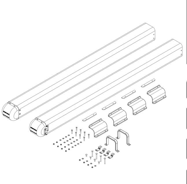
SPLICED CONDUIT TUBE ASSEMBLY
