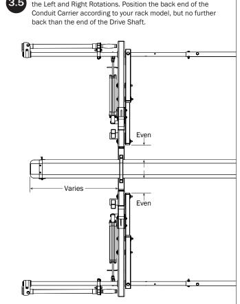
Center the front and rear of the Conduit Carrier evenly between
