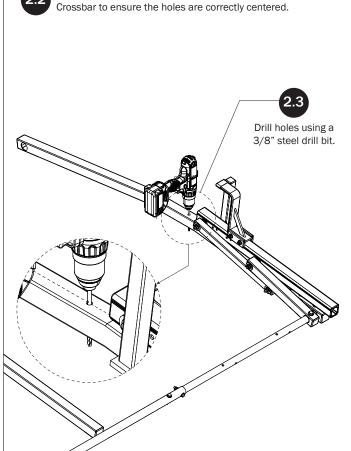
Prior to drilling, mark a center line along the length of the
