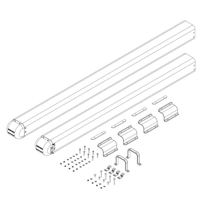
SPLICED CONDUIT TUBE ASSEMBLY
