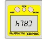
(4) Rotate 90 degree clockwise, hold the instrument and keep it still, press the "ZERO" button again, the LCD displays "CAL5";
