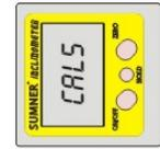
(5) Rotate 90 degree clockwise, hold the instrument and keep it still, press the "ZERO" button again, the LCD displays "PASS"; then displays "0.00"
