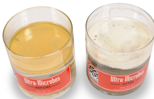
Test samples: Container on left shows untreated oil and water. Container on right was treated with Ultra-Archaea and shows only lipids that were left after the bio-remediation took place.
