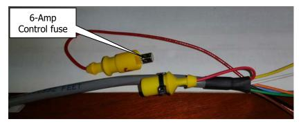
Gently pull the fuse holder apart as shown. Note that end with the black wire tie is designed to say in place tied to the cable.
