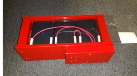
2. Remove the four corner screws that hold the clear cover on, and slide the cover off.
