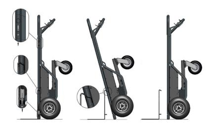
Flat Plate Attached and Locked.
