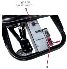
Auto return to zero from forward or reverse will slow down and stop the unit if contact with throttle is lost.
