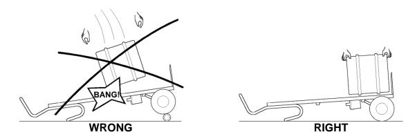
During normal operations, the battery is held securely in place by locking hooks. A strong, vertical pull is required to remove it. Moving backwards very quickly and striking a high step or similar equipment abuse could result in the battery ejecting from its location. If this happens, the Powered Stair Climber will cease operation. Failure to negotiate steps "square-on" will damage the underside of the drive unit.
