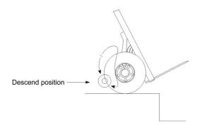
With the support wheels in the descend position, the Powered Stair Climber can be rolled over the step and the support wheels will lower the Powered Stair Climber onto the next step down. When the main wheels land on the lower step, the support wheels automatically rotate to the descend position for the descent onto the next step, all within approximately half a second.
