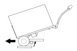
Press ascend / descend button briefly again until the indicator light flashes green. The Powered Stair Climber is now in the descend mode and the support wheels will move to the descend position automatically. The round up switch is now non-functional.
