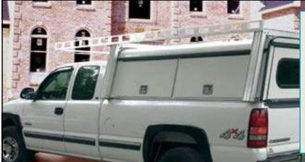
System One's Cantilever Mounts allow the Contractor Rig® to be installed over truck caps. Our in stock sizes fit most caps; others can be cut to order. The stainless steel mounts are fastened to the structural Pick-Up Trak®, instead of to the thin sheet metal of the bed rail. This mounting method distributes the weight evenly on the bed rail resulting in an extremely rigid installation.
