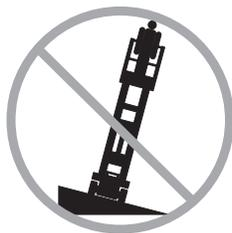
Do not depend on the tilt alarm as a level indicator. The tilt alarm sounds at the platform controls and the ground controls when the machine is on a severe slope.
