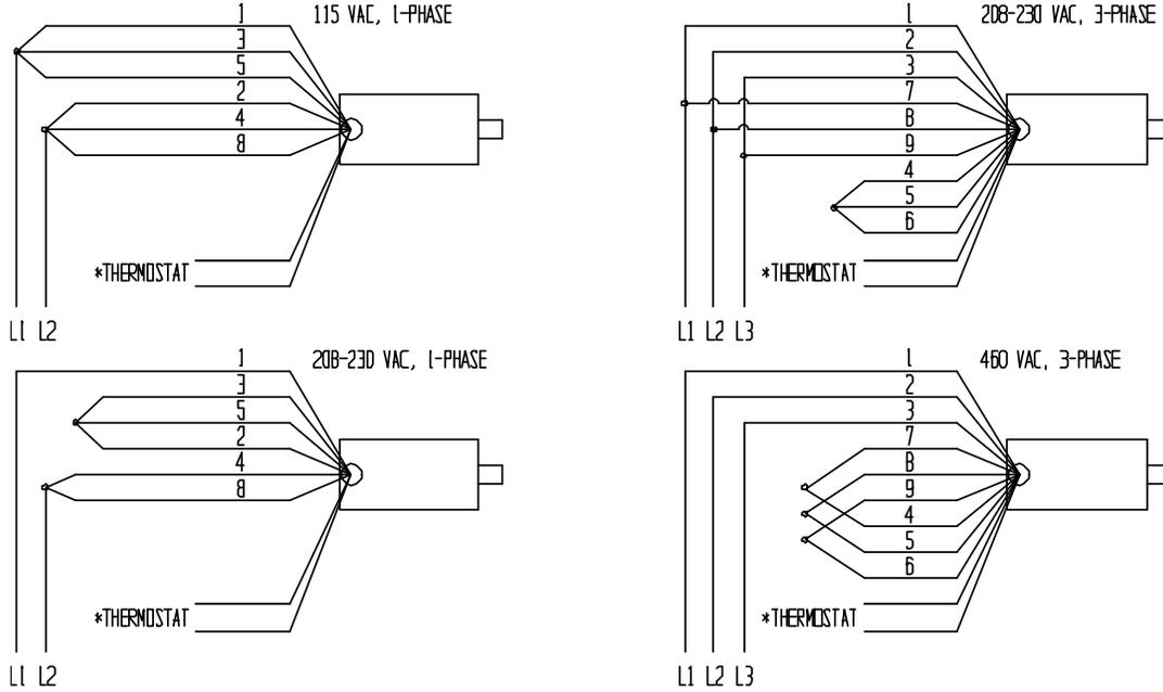
\* The two thermostat leads go to: 1) the grounded side of the transformer secondary, and; 2) the motor relay coil, in either order.
