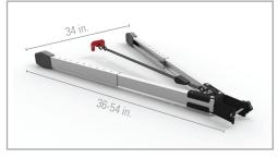
**EXTENDABLE V-BRACE** The Extendable V-Brace, when retracted, is the same size as the standard V-Brace, and can move in 2 in. increments and expand to 18 in., creating a total wall distance of 51 in.
