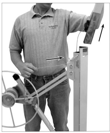
3. Remove the two telescoping sections completely from the frame housing. Pull the cable completely out from the frame along with them. BE CAREFUL for loose strands or frays on the cable.
