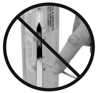
**DO NOT** feed the cable under the cable sheave on the frame as shown in this photo!
