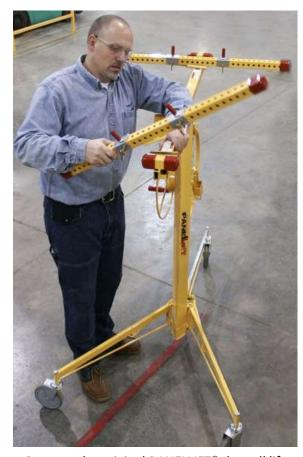
Remove the original PANELLIFT® drywall lift cross arms and attach the HVAC cross arms as shown.
