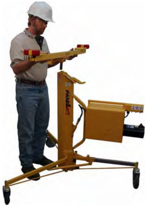
10. MOUNT THE CRADLE ON TOP OF THE TELESOPING SECTIONS. PULL OUT ON THE TILT LATCH TO ALLOW THE CRADLE TO TILT FOR LOADING AND FOR HANGING DRYWALL ON SIDEWALLS AND SLOPED CEILINGS.
