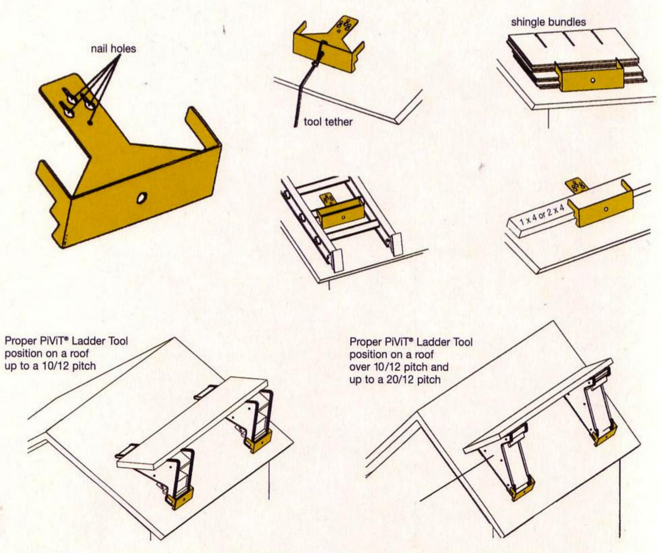
RoofBoot™ shown here being used with the PiViT® Ladder Tool.
