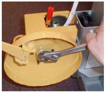
8) Install the winch nut and fasten securely in place. (You will find it helpful to lock the winch from rotating while tightening the winch nut by carefully inserting a small screw driver into the gear mechansm.)
