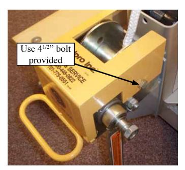
4) Install the winch guard and fasten in place with the  $4^{1/2}$ " Bolt and lock nut provided for the winch spool axle bolt. (The bolt removed in step 3 above will be too short.)
