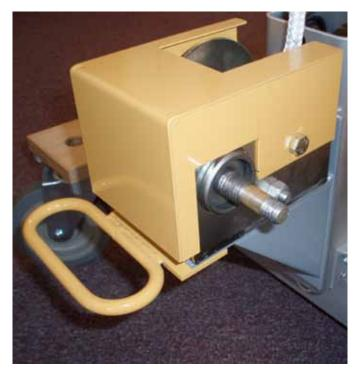
5) Remove the standard winch Nut and Spring. Remove handle by rotating counter clockwise. (You will find it helpful to lock the rotation of the winch by carefully inserting a small screw driver into the gear mechanism)
