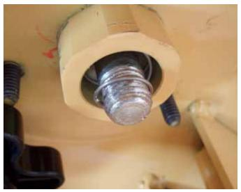
7) Install the winch handle spring as shown with the wide end in first and the narrow end out.
