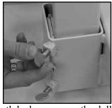
2. Tighten both lock screws on the dolly base to hold the boom tube securely.
