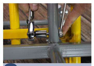
Screw a 5/16" nut onto the bolt and tighten down with a **1/2" wrench and socket**. Repeat for the other three bars.
