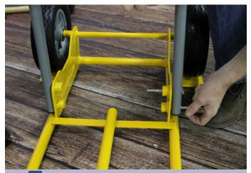
Insert two bolts 5/16" bolts (3-1/2"L) through the rear wheel assembly and cart frame. Repeat on other side. DO NOT install the nuts at this time.
