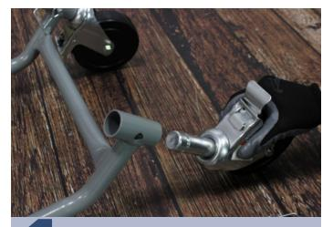
Insert the caster into the rear wheel assembly.
