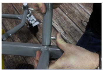
Insert a 5/16" Hex Head Bolt (1-1/2" L) through the holes on both the front and rear chair bar.
