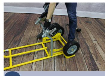
Align the rear wheel assembly over the holes on the back of the cart.
