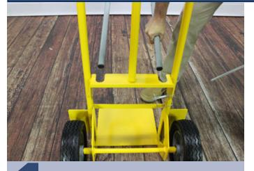
Remove the hair pin from the clevis pin that holds the chair bar in place.
