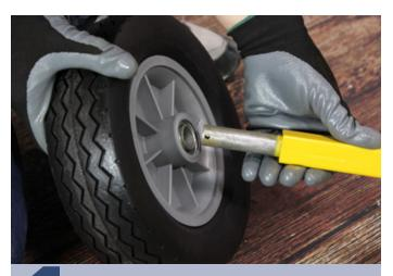
Slide the first wheel onto the axle, making sure the offset side of the hub goes towards the body of the cart.
