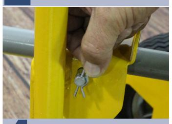
Secure the clevis pen in place with the hair pin.
