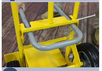
Insert the clevis pin through the holes on the chair bar.
