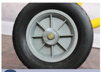
Slide the washer onto the axle.
