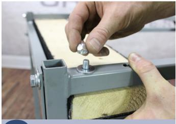
Slide the bolt through the cart frame and carpeted wood. Secure with a 5/16" washer and 5/16" nylon locknut.
