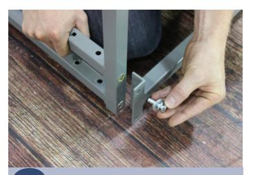
Align the bottom frame piece to a side frame piece.
