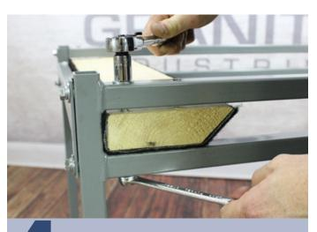
Tighten down using a 1/2" socket. Repeat steps 1-3 for the remaining holes.
