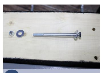
Slide a washer onto the 4"L 5/16" bolt.
