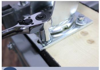
Tighten the bolts down using a 1/2" socket. Repeat steps 1-2 for the remaining casters.
