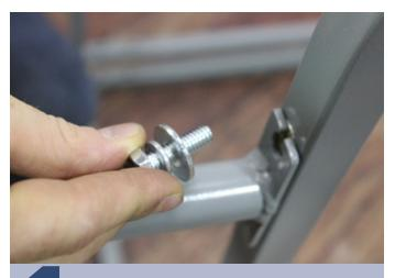
Align the handle over the holes. Slide a lock washer and a washer onto the bolt and insert into the hole.
