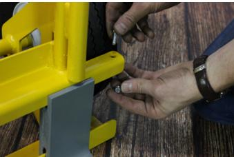
Insert the 1/4" hex bolt into the hole and secure it with the 1/4" lock nut.
