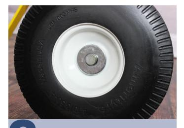
Slide the washer onto the axle.
