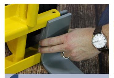
Slide the fork onto the cart frame as shown. Repeat for the other side.
