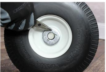
Insert the cotter pin and secure it by bending both ends outward with a **needle nose pliers**.
