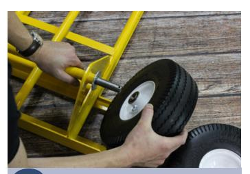
Slide a 3/4" washer, and a wheel onto the axle, making sure the offset side of the hub goes towards the body of the cart.
