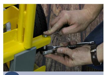
Tighten down using a **7/16" wrench and socket**.
