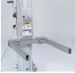
ADJUSTABLE FORKS widen from 11 to 30 in (28 to 76 cm) to accommodate diverse loads.
