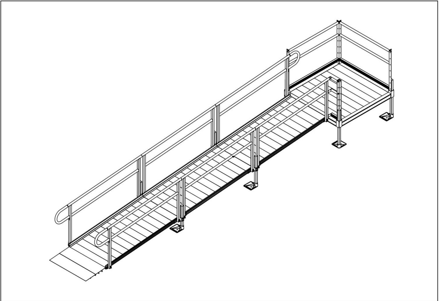
**Configuration shown with straight ramp run and 4' x 4' top platform.
