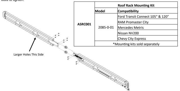
STEP 3. Insert (2) Connecting Caps into Front Right End Rail (larger holes on the bottom outside). With the larger holes on the bottom outside, slide the Rear Right End Rail over the other end of the caps. Assemble together using (4) 5/16-18 x 5/8" carriage bolts, washers, and nylon lock nuts. Tighten to 150 in-lb or 13 ft-lb. Do NOT use impact tools to tighten.
