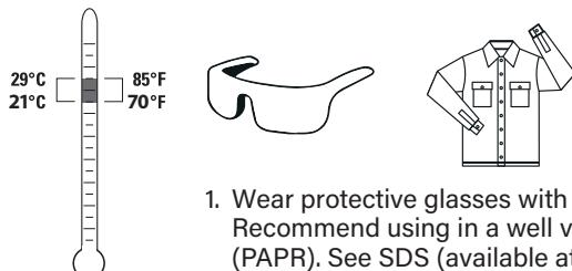
1. Wear protective glasses with sideshields or goggles, nitrile gloves, and clothing that protects against dermal exposure. Recommend using in a well ventilated area with certified respiratory protection or a powered air purifying respirator (PAPR). See SDS (available at [www.sealsprayfoam.com](http://www.sealsprayfoam.com)).
