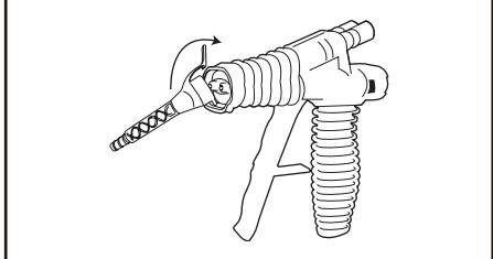
2. Insert bottom tab of nozzle into bottom slot of dispensing unit.
