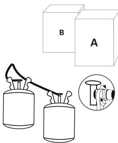
3. Thread **RED CODED HOSE TO A-COMPONENT CYLINDER** and **BLACK CODED HOSE TO B-COMPONENT CYLINDER** and tighten with supplied 9/16" wrench.
