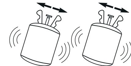
2. Shake each cylinder for one (1) to two (2) minutes to ensure proper mixing. Chemical should be between 70-85°F (21-29°C).
