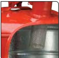
Stainless steel flame arrester stops flashback ignition. Long 3-1/2" (88-mm) length offer safe secure insertion of gas nozzle.
