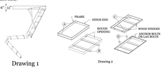
A. Pre-drill holes in frame (Drawing 2), 2 in the hinge end and 2 in the sides on the opposite end.
